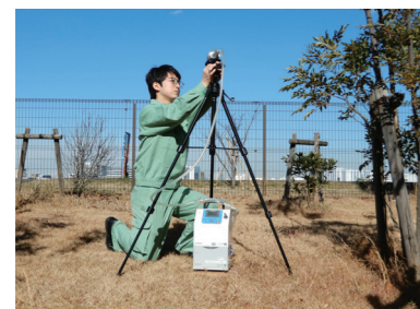
Collecting asbestos in the air
