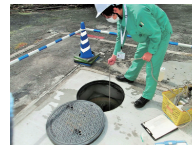
Sampling drainage at an operational facility
