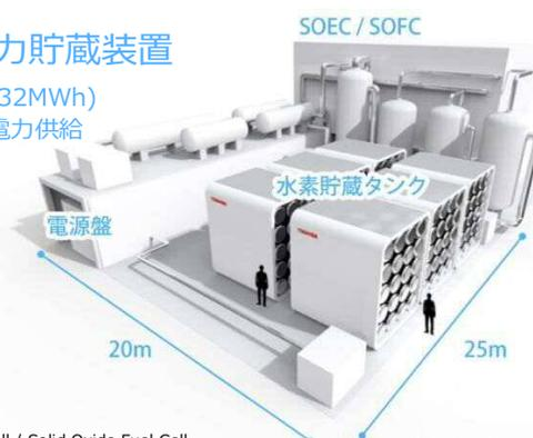
\*SOEC/SOFC : Solid Oxide Electrolysis Cell / Solid Oxide Fuel Cell
