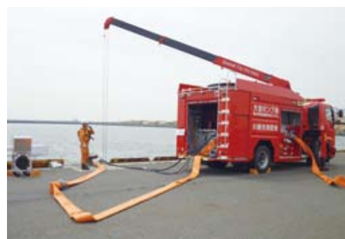
災害時に大量の海水等を利用して消火できる大型ポンプ車 Large-scale pumping vehicle used to extinguish fires with large amounts of sea water, etc. in the event of disasters
