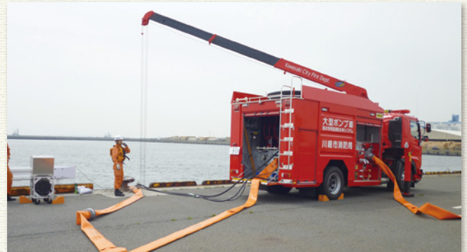
災害時に大量の海水などを利用して消火できる大型ポンプ車 Large-scale pumping vehicle used to extinguish fires with large amounts of sea water, etc. in the event of disasters
