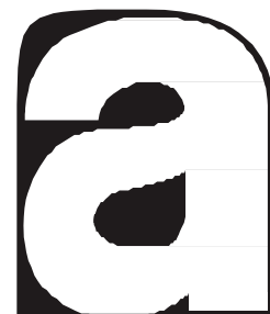
Asbestos mark (Construction materials containing asbestos)
