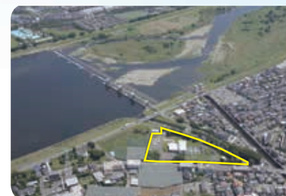
Inada Intake Station River water of the Tama River diverted to the Nikaryo Reservoir by the Kamigawara Dam is taken at the Inada Station.
