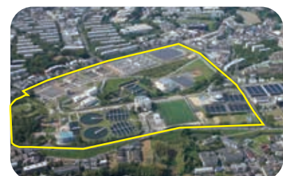
Nagasawa Purification Plant Started passing water in June 1954. The original water is river water from the Sagami River, the treatment method is coagulation sedimentation process, and the water supply capacity is 235,000 m 3 /day. A regulating reservoir and other facilities were constructed under the Restructuring Plan.
