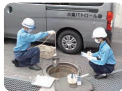
Wastewater sampling at business sites
