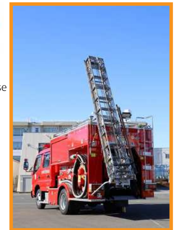
The triple ladder has a tilted stand that makes it easier to access.
